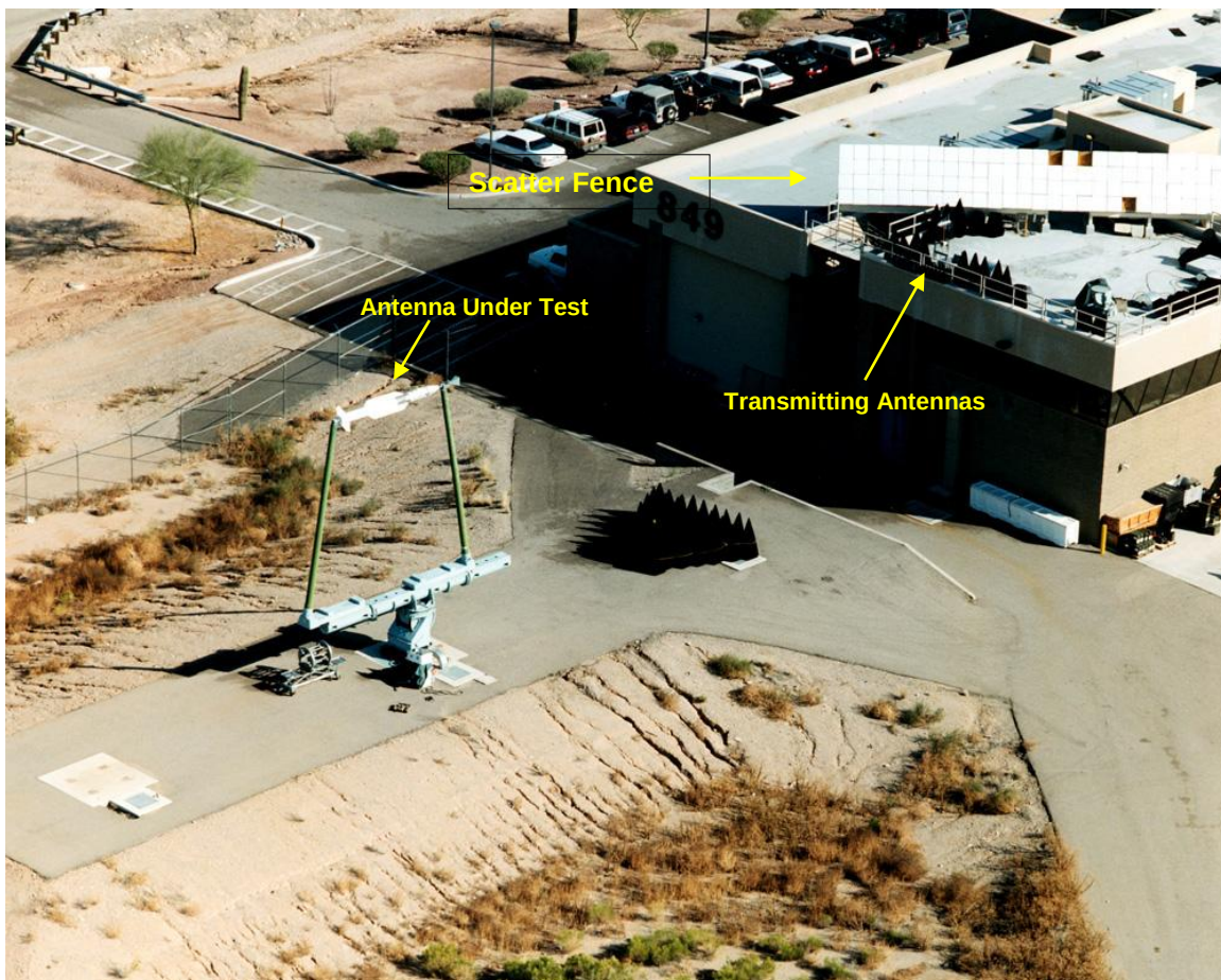
Figure 2: Outdoor Antenna Test Range
