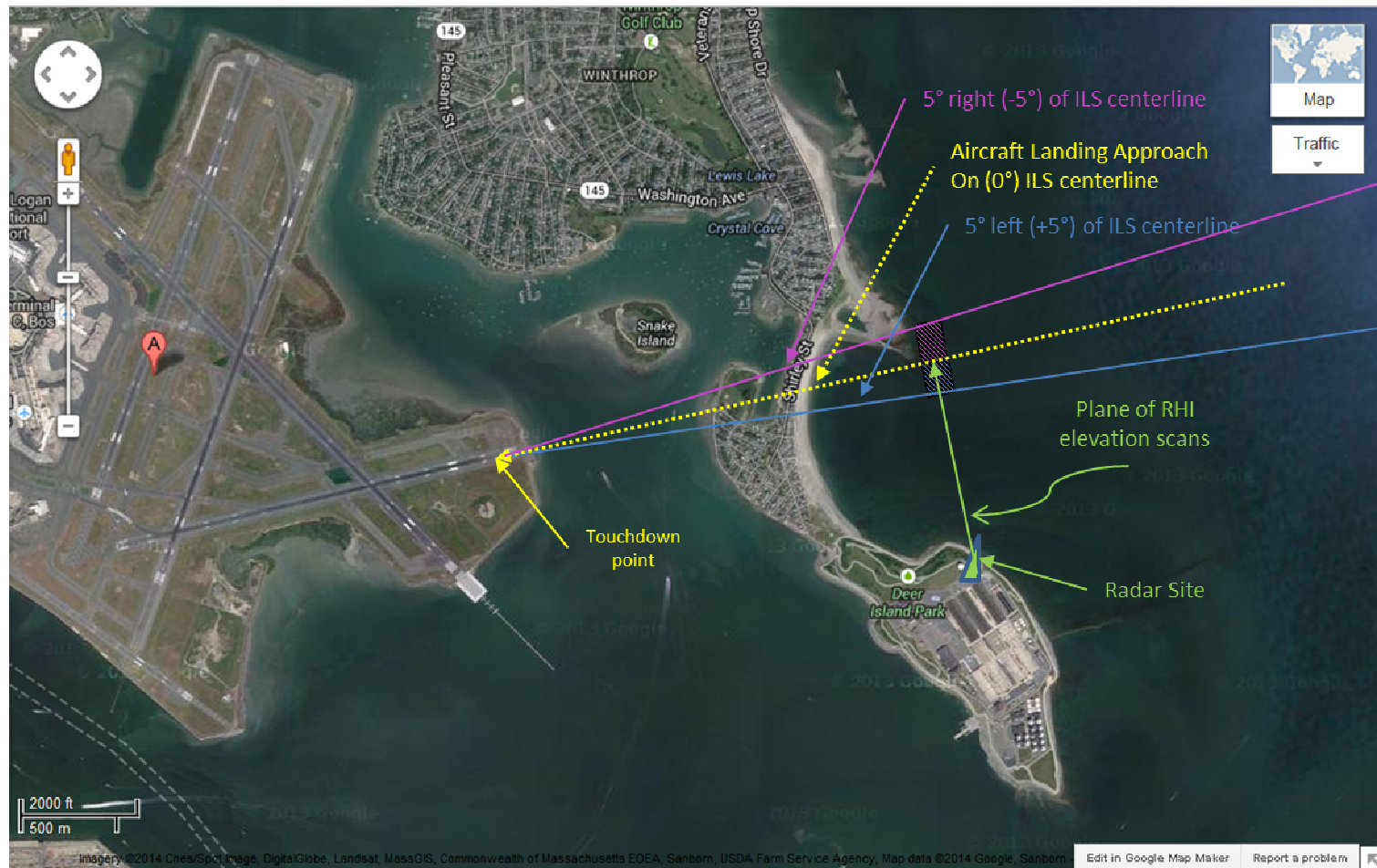
Figure 2: Radar on Deer Island to Observe Aircraft Approaching Boston Logan RWY 27
