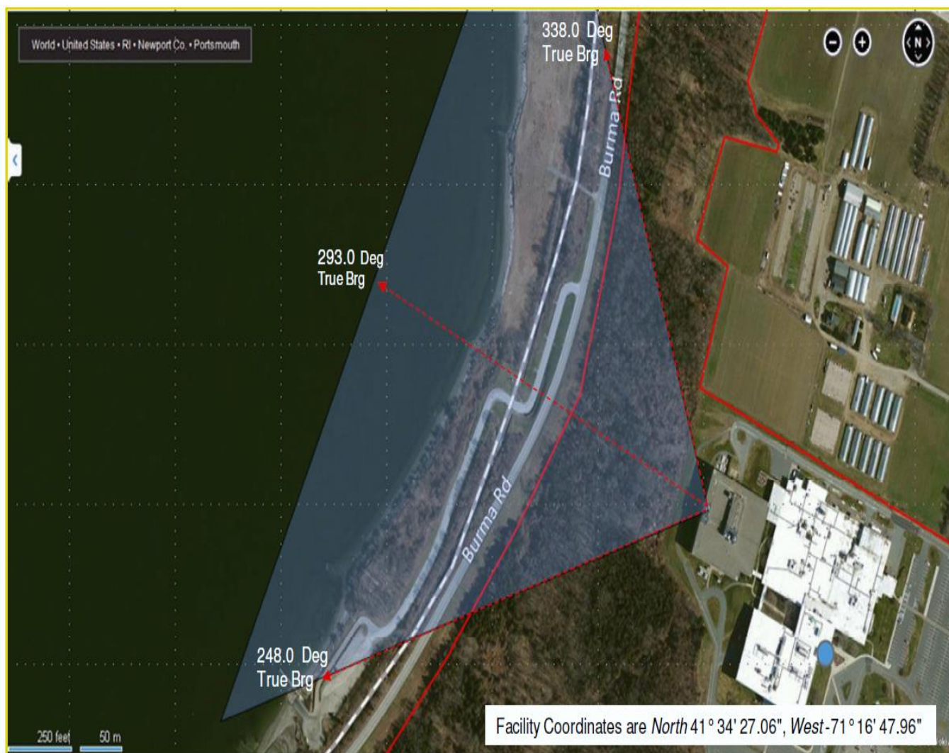
Figure 2. Portsmouth, RI Test Facility. This graphic depicts the location of the radar at the test facility, as well as the intended azimuth coverage area and direction of radiation (Blue Shaded Area). The solid Red lines define the fenced boundaries. The dotted Red lines define the Radiation Boundaries.
