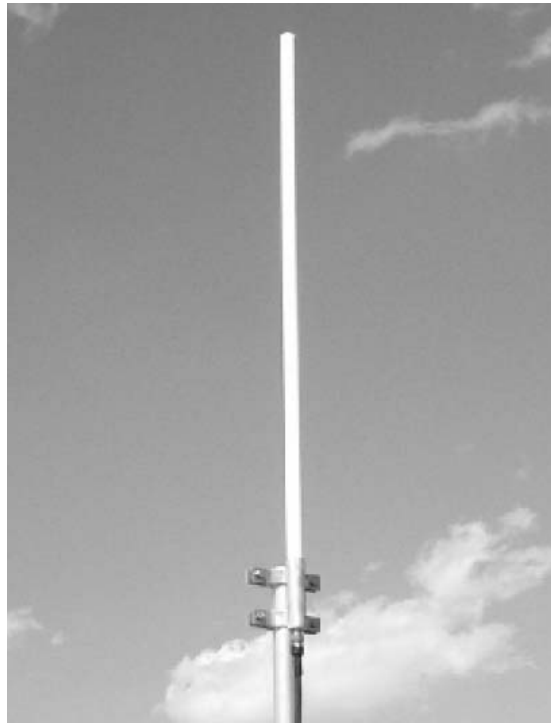
Figure 3 : Omni directional antenna element (L =135 cm)
