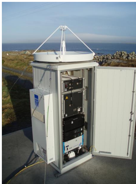
Fig. 2: Samples of vertically pointing cloud radar MIRA-35 installed in an outdoor enclosure for vertical pointing (left) and in an outdoor enclosure with positioner on top (right). In both enclosures the radar components are installed in a 19" rack and are operated in a temperature controlled or air-conditioned environment.
