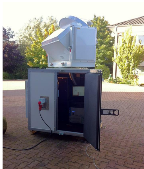
Fig. 2: Samples of vertically pointing cloud radar MIRA-35 installed in an outdoor enclosure for vertical pointing (left) and in an outdoor enclosure with positioner on top (right). In both enclosures the radar components are installed in a 19" rack and are operated in a temperature controlled or air-conditioned environment.
