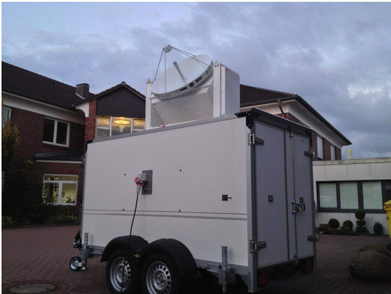
Fig. 1: MIRA-35 with scanning unit mounted on top of an enclosed trailer. The radar components and the antenna (here: \varnothing 1 m) are mounted on a two-axis positioner.
