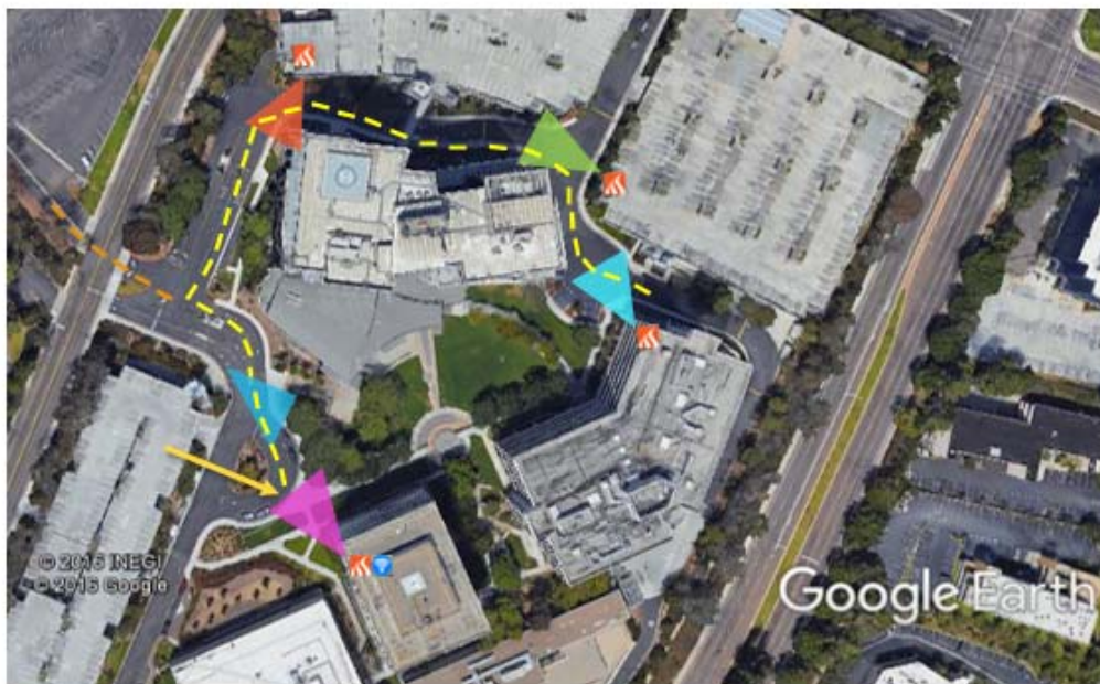
Figure 2 Directional Antenna Orientations
