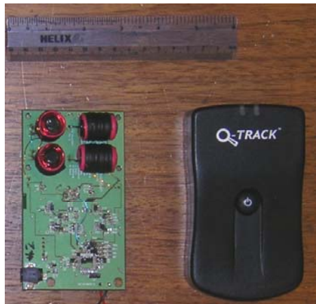
Q-Track QT™-400 tag transmitter prototype with four element antenna array.
