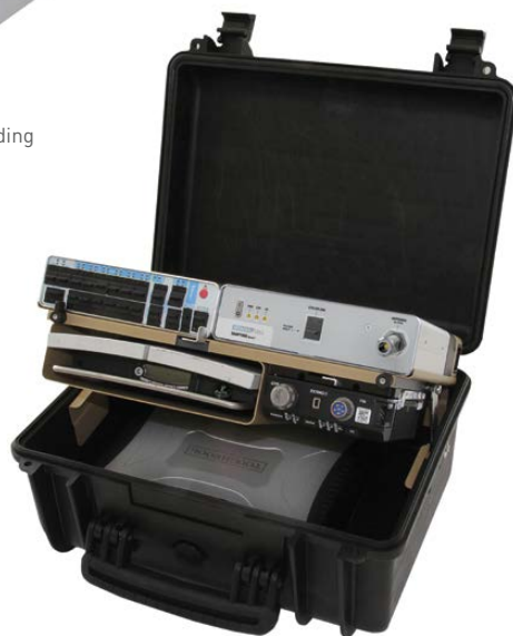
VoyagerCell in Voyager Express transit case with Inmarsat BGAN terminal and laptop
