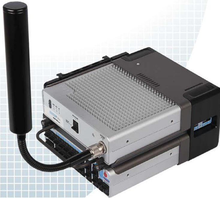
VoyagerESR and 3GAP1000 radio node packaged in Voyager 2 chassis
