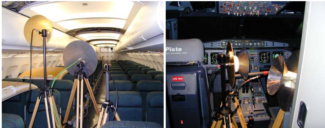
FIGURE 27 - ANTENNA SET-UPS FOR CABIN AND COCKPIT TESTS
