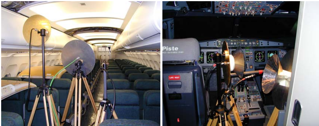
FIGURE 27 - ANTENNA SET-UPS FOR CABIN AND COCKPIT TESTS
