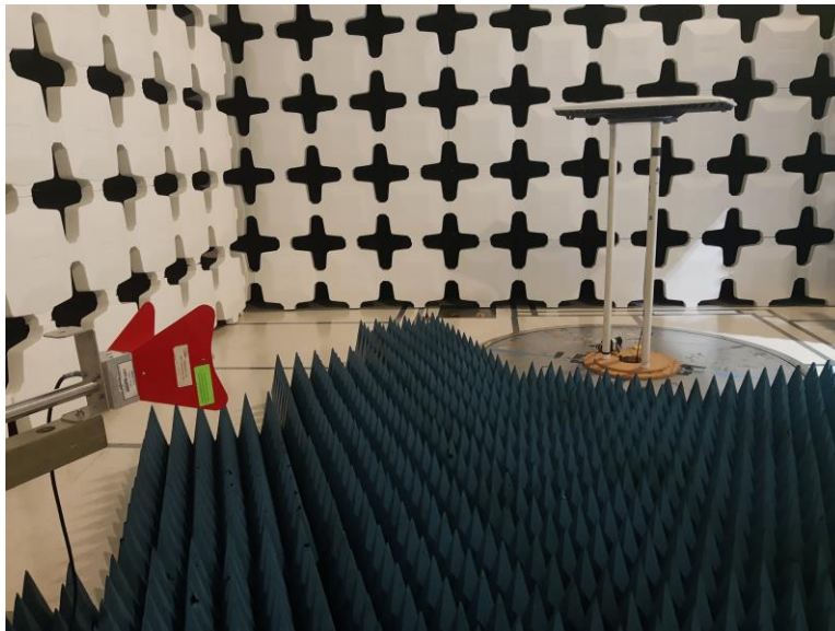
Photograph 3. RE Setup [1 GHz - 18 GHz]
