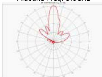
Elevation Radiation Pattern Midband Freq. 3.6GHz
