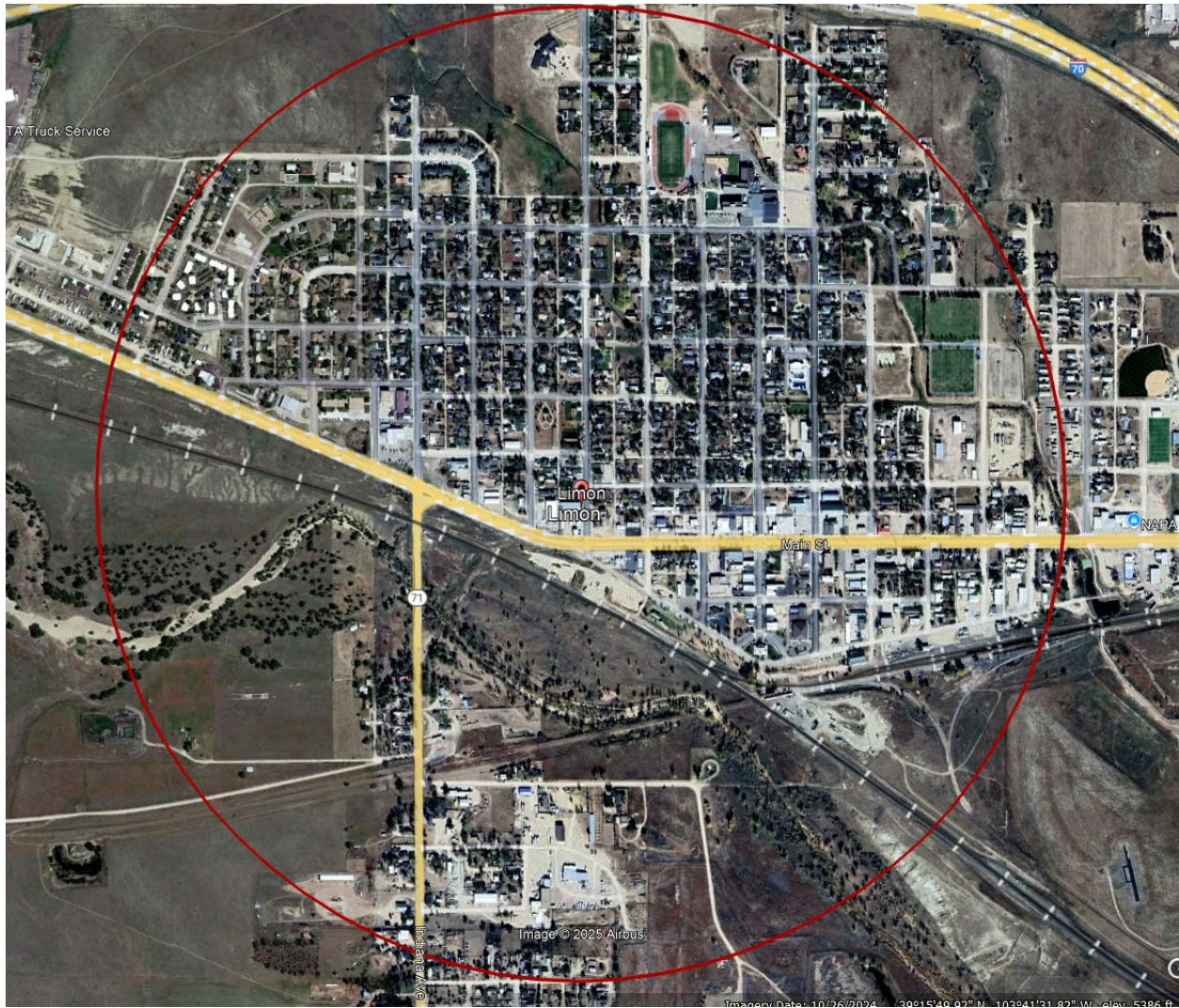
Figure 6: Limon Installation. The red circle represents a 1 km radius around the center point, and the transmitter will be moved within that area to optimize operations. Lat. 39-15-50 N, Long. 103-41-32 W
