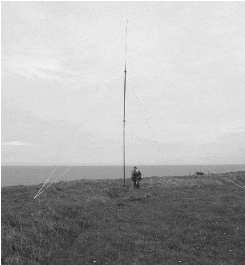
Photo: showing 12m (vertical height) transmit antenna.
