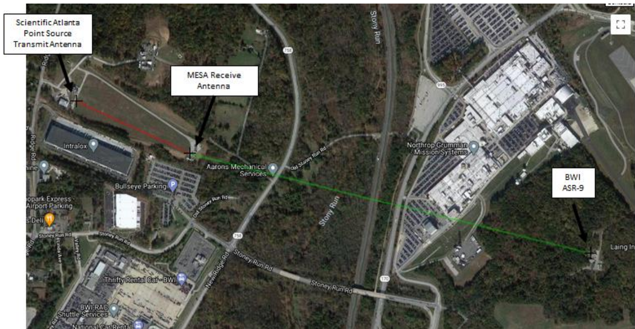
Figure 1 – Antenna Range Point Source to BWI ASR-9 Antenna Geometry
