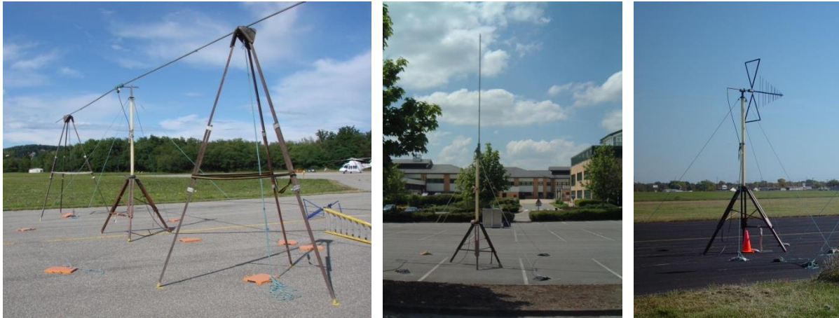
Figure 2 - LLSC Antennas - HF Dipole Horizontal & Vertical and BiLog Vertical
