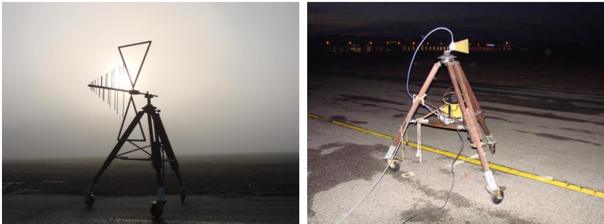
Figure 6 - LLSF antennas - BiLog and Double-Ridged Guide Horn
