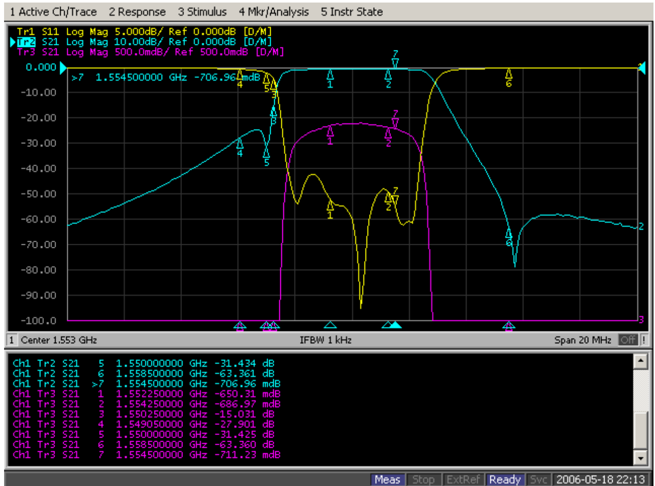
Figure 2: Cavity Filter Characteristics
