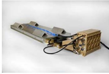
Figure 2: Miniature Localizing Ground Penetrating Radar
