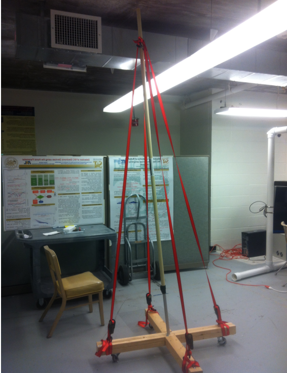
Figure 1: Transportable tower for gateway node.
