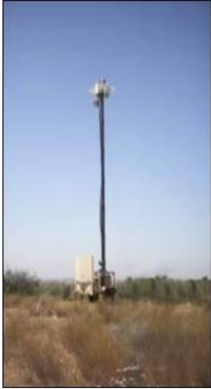
This antenna unit can be telescoped to approximately 16 meters.
