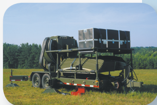
The system shown here features a 16-panel 5.4 meter reflector, a high performance autotracking X-band feed, as well as Y-over X-axis pedestal configuration.
