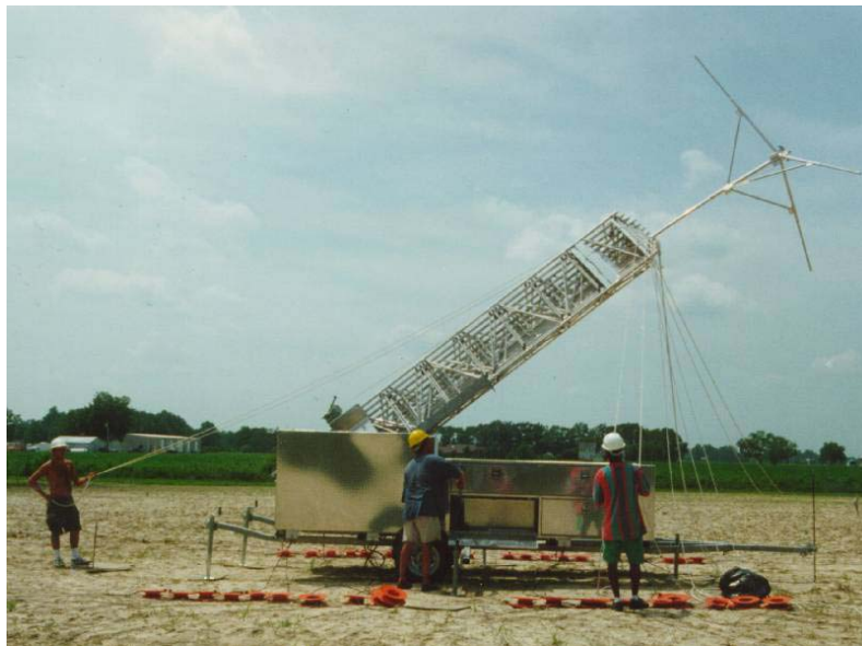
Figure 1: The TUP-3 Antenna being deployed for experimental field tests.
