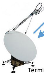
Terminal #1: Hawkey III 2.4 m Parabolic Reflector Antenna C-band EIRP: 57.3 dBW X-band EIRP: 60.8 dBW Ku-band EIRP: 63.8 dBW Ka-band EIRP: 65.2 dBW (commercial) Ka-band EIRP: 69.5 dBW (U.S. Military)
