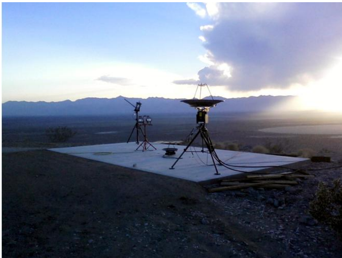
Figure 2 Typical Deployment of NVDF Calibration System Antennas
