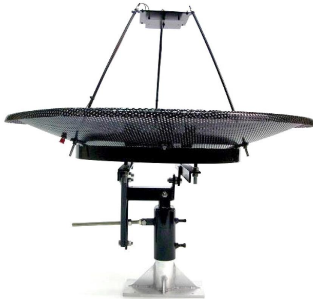
Figure 1 NVDF Calibration System Antenna on Test Mounting Base
