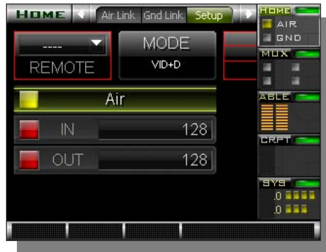
Figure 3-42. C100 Controller MUX Ground to Air Page
