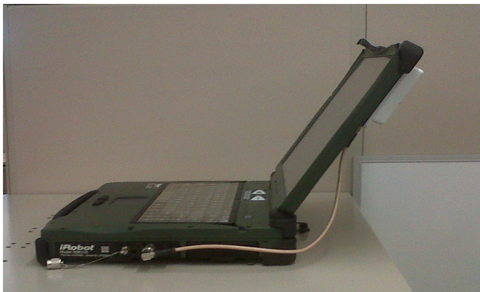
Illustration 2: Minimum operational antenna angle
