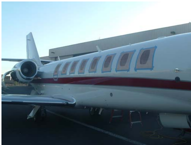
Figure 5. Shielding material fixed to aircraft
