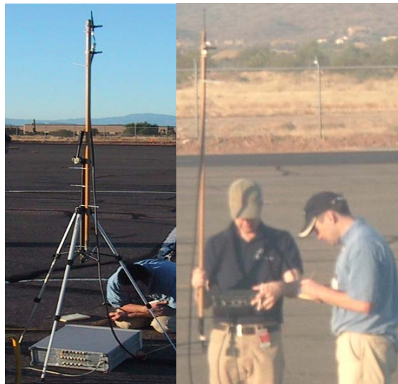
Figure 12. Transmitter and Receiver set-up for baseline tests
