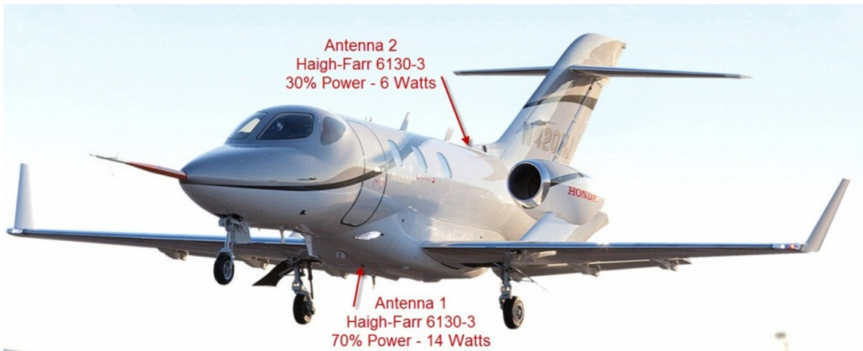
Figure 3 - Telemetry Antenna Arrangement
