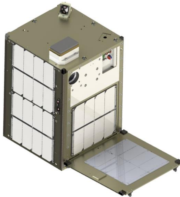
Figure 1 1HOPSat-TD 12U Satellite Configuration, Deployed
