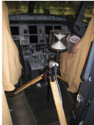
Figure 1; example of test antenna at flight deck position
