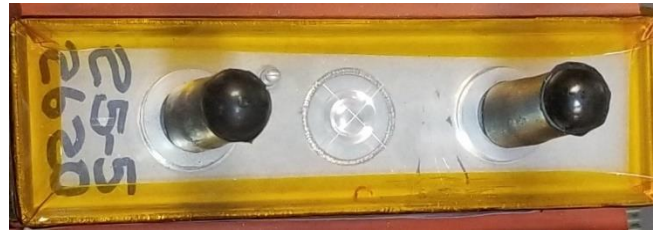
Figure 9: Battery Burst Disk
