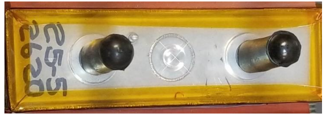
Figure 9: Battery Burst Disk
