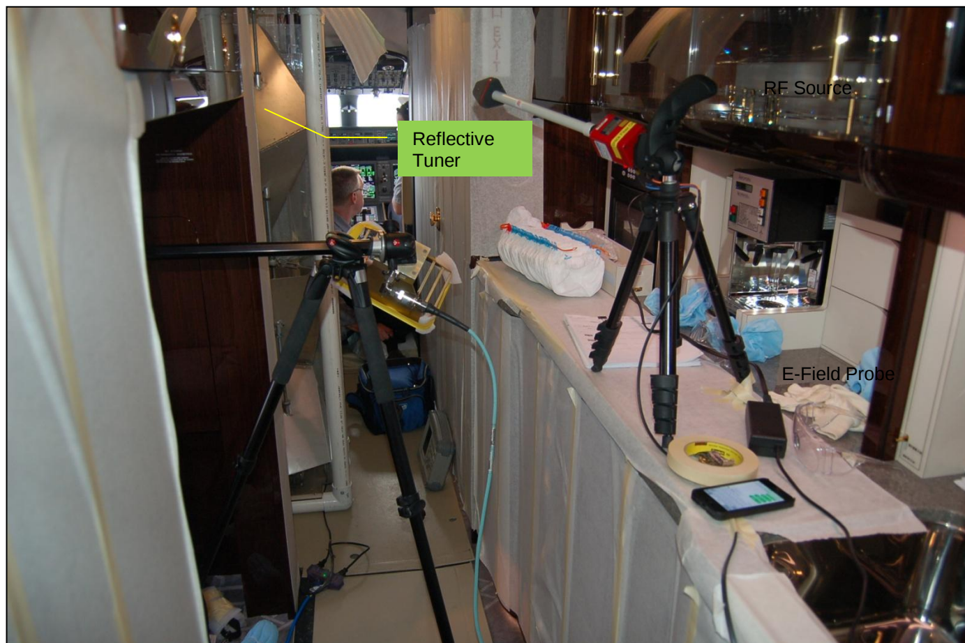
Photo 1: Sample TPED Test Arrangement
