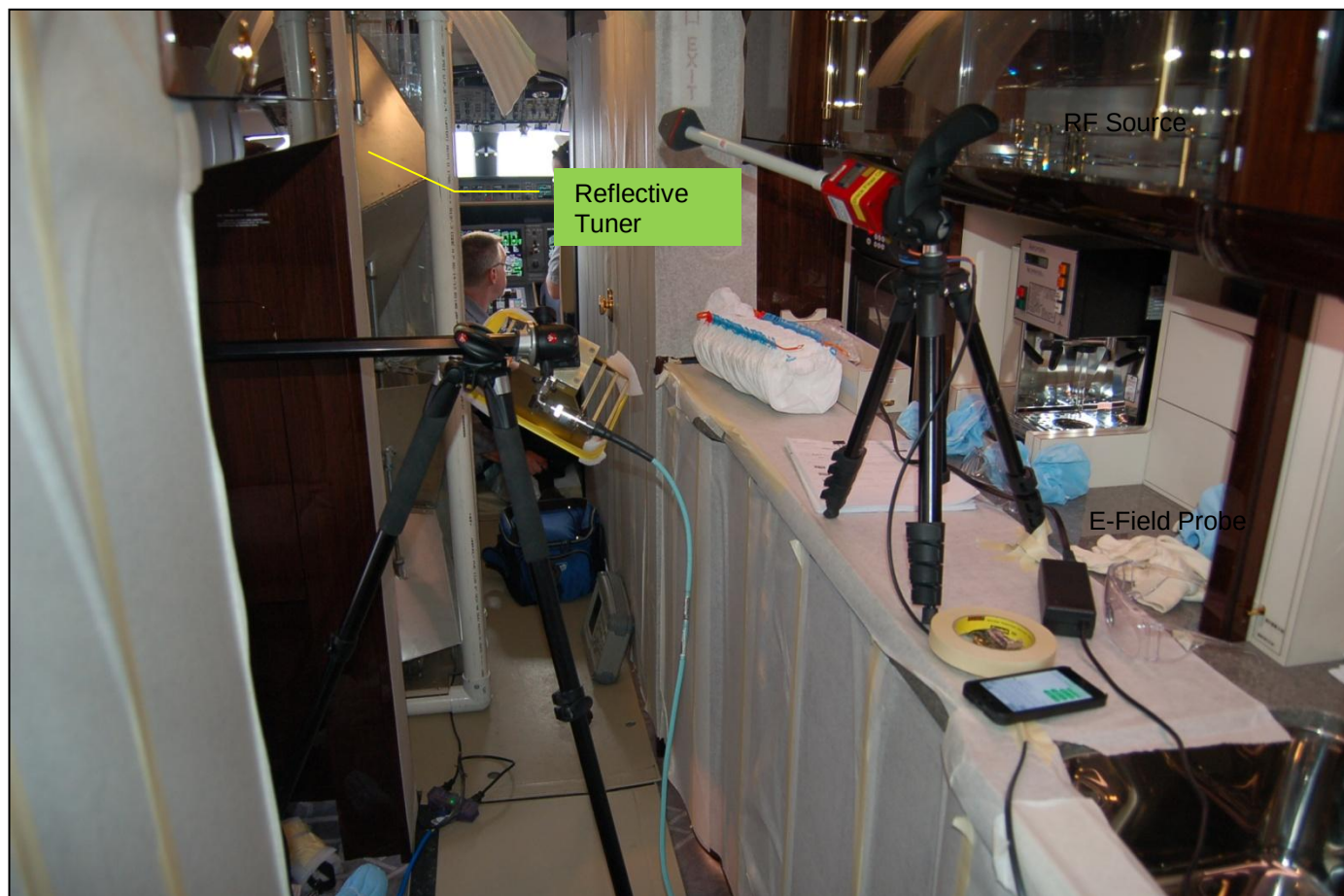
Photo 1: Sample TPED Test Arrangement
