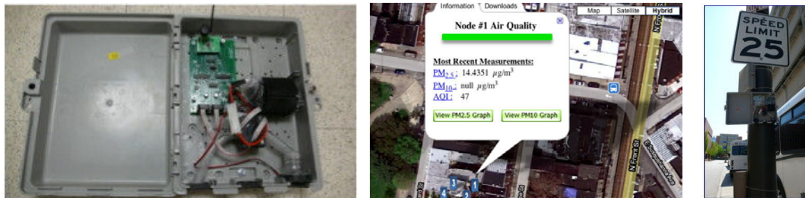
Figure 2: Illustration of (a) Custom-built sensor packages interfaced with ZigBee radios, (b) Picture of the environment in which air quality simulations and sensor deployment were performed, and (c) Actual deployment of a sensor in the environment.
