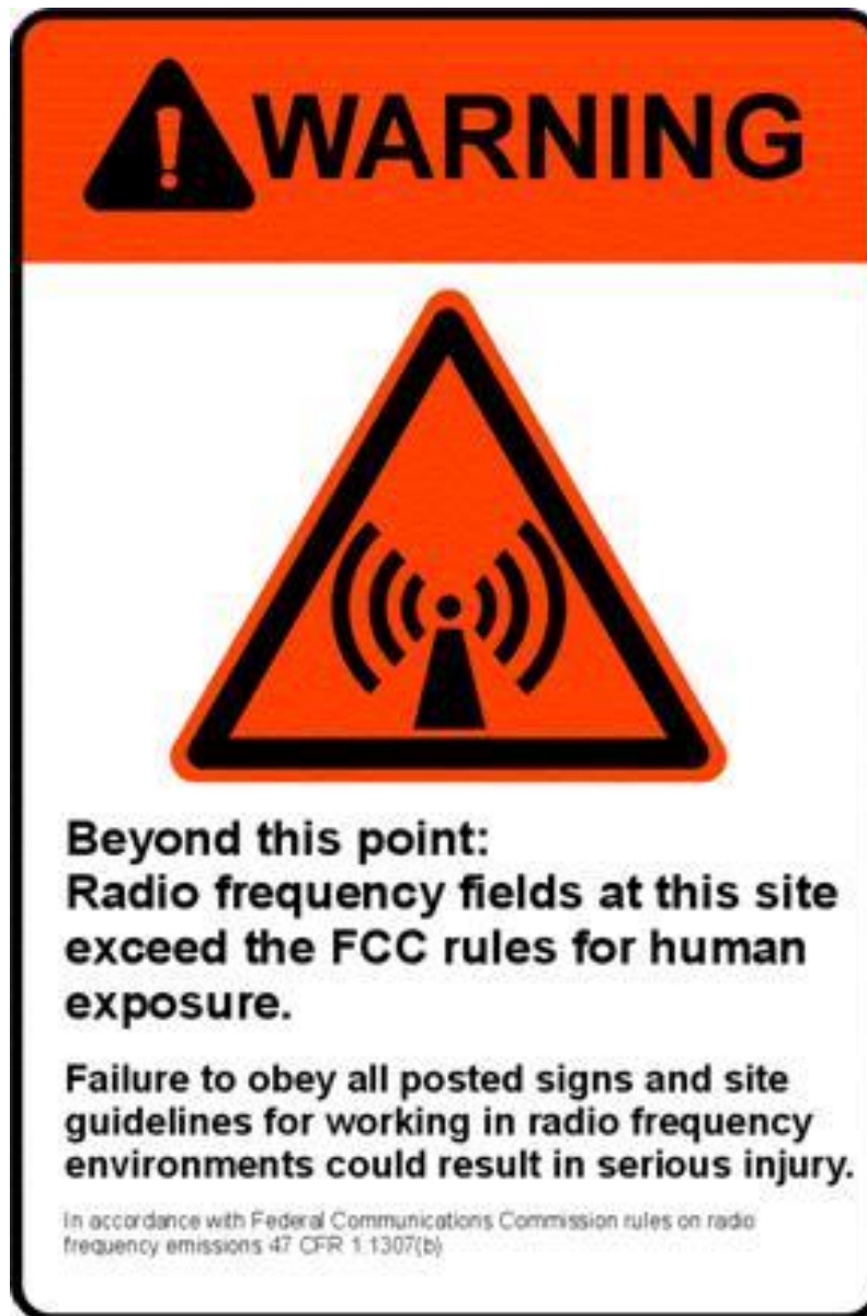
Figure 2 - Radiation Hazard Warning Label Sample
