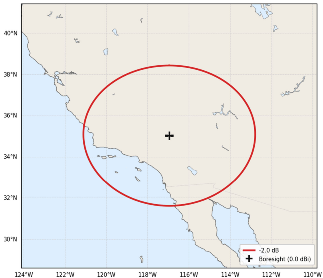
Figure 4. UUA Antenna Beam Projection over SG_RANCH from Orbit altitude of 510 km
