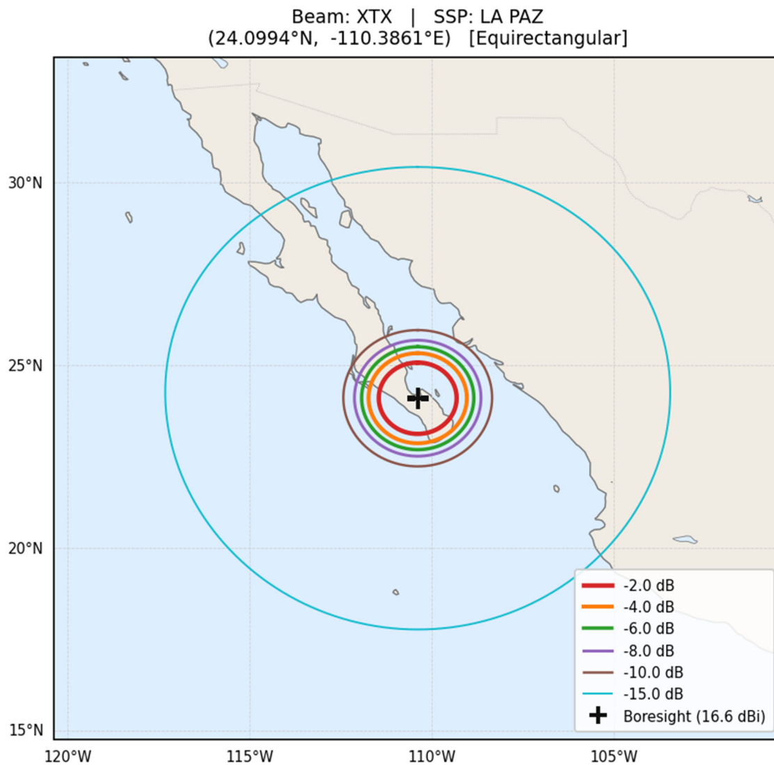
Figure 26. XTX Antenna Beam Projection over LA PAZ from Orbit altitude of 510 km
