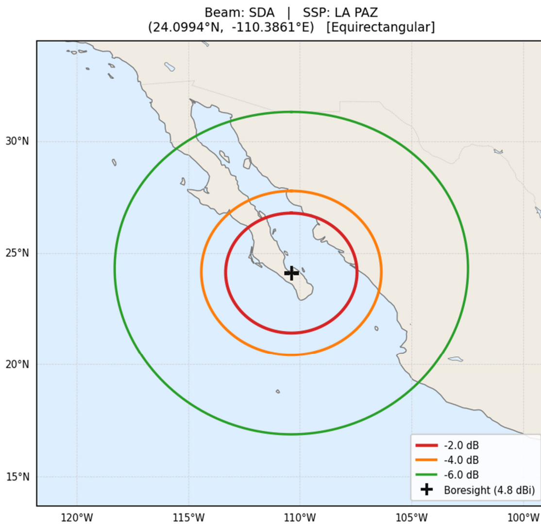
Figure 8. SDA Antenna Beam Projection over LA PAZ from Orbit altitude of 510 km
