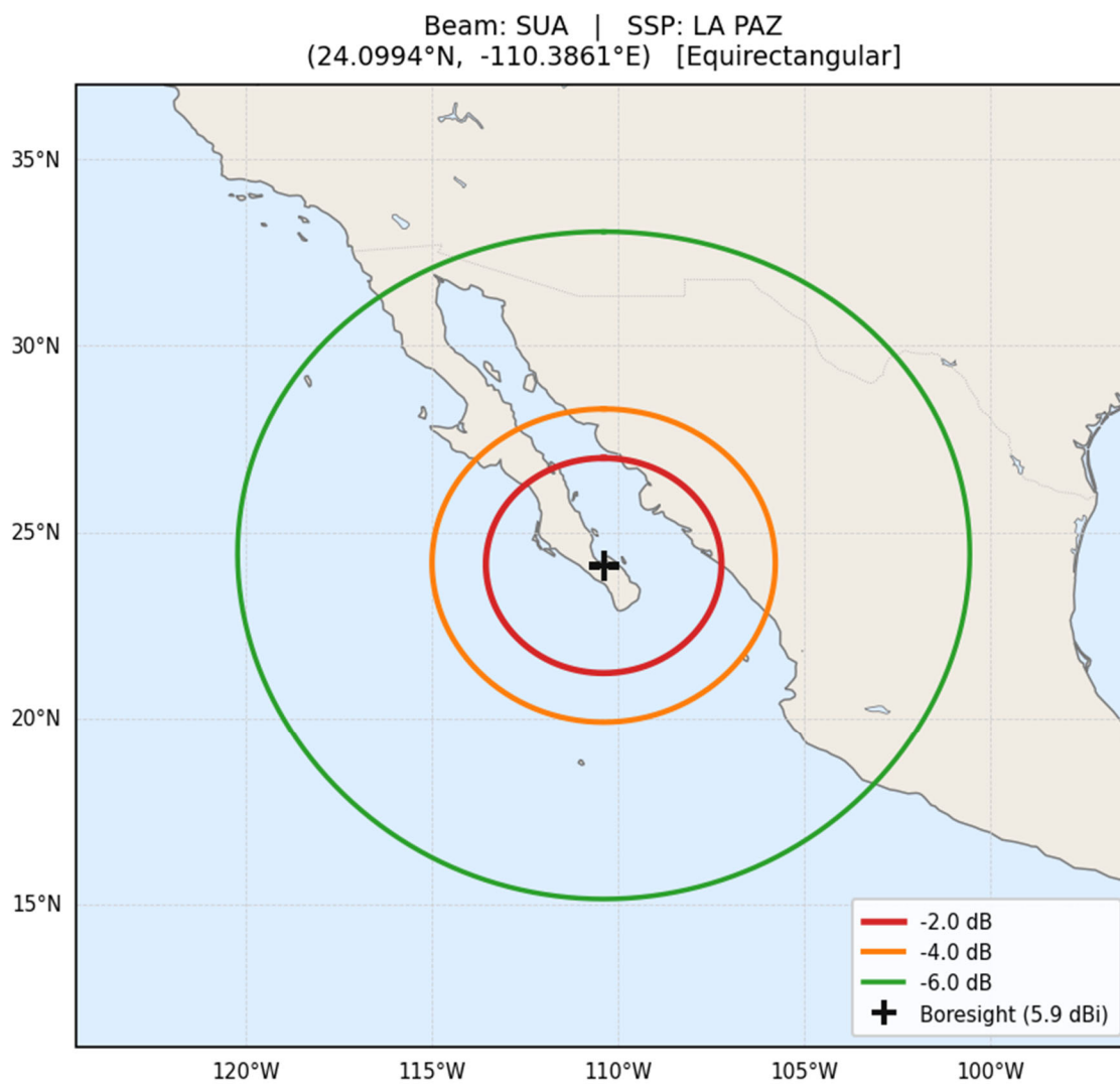
Figure 15. SUA Antenna Beam Projection over LA PAZ from Orbit altitude of 450 km
