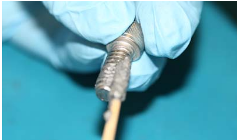
Figure 3.4 Applying the Anti-Seize Lubricant
