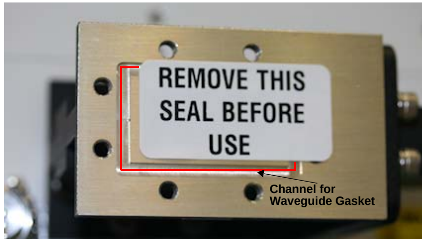
Figure 3.5 Waveguide Label and Channel for Gasket
