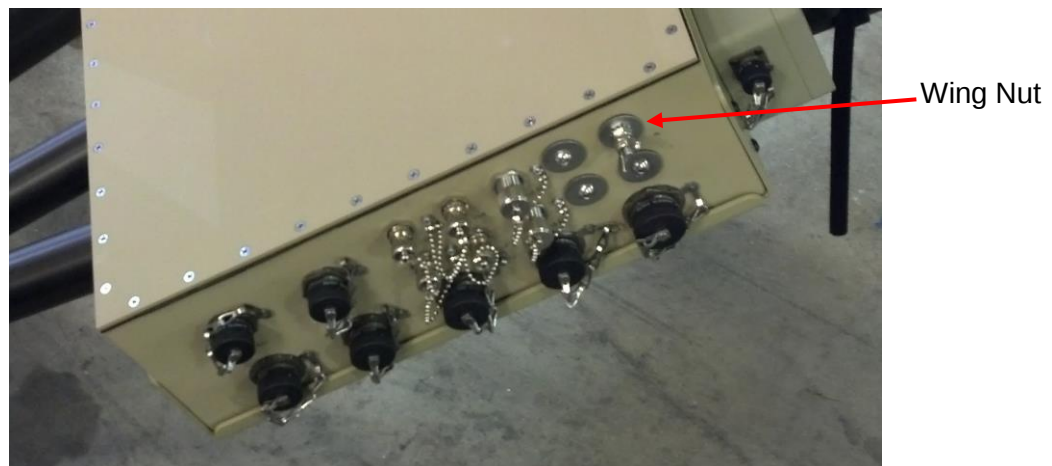
Figure 42. Grounding Wing Nut on RC4000
