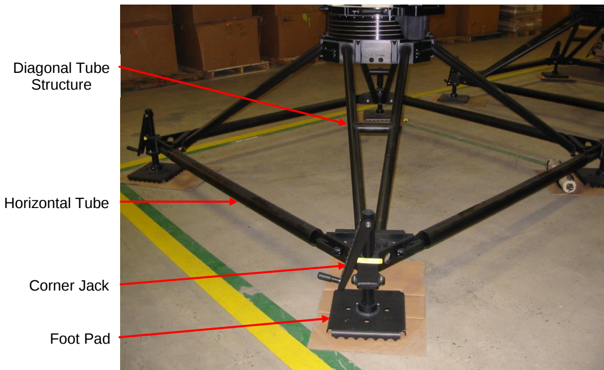
Figure 12. Completed Quad-Pod Assembly
