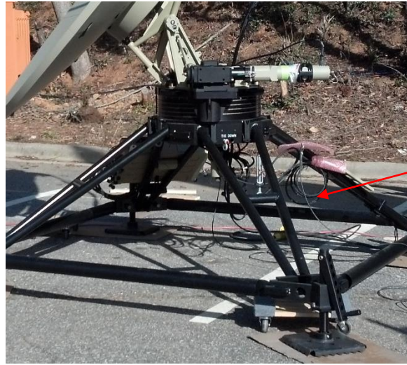
Figure 73. Wiring Bundles on 2460 HW Cont.
