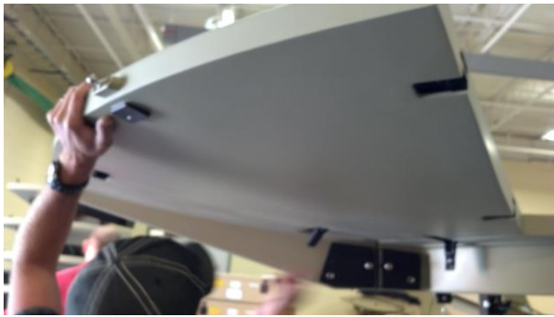
Figure 22b & 22c. Attachment of Reflector Panels 2 and 8
