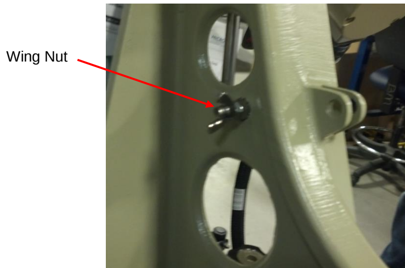
Figure 41. Grounding Wing Nut on Elevation Frame
