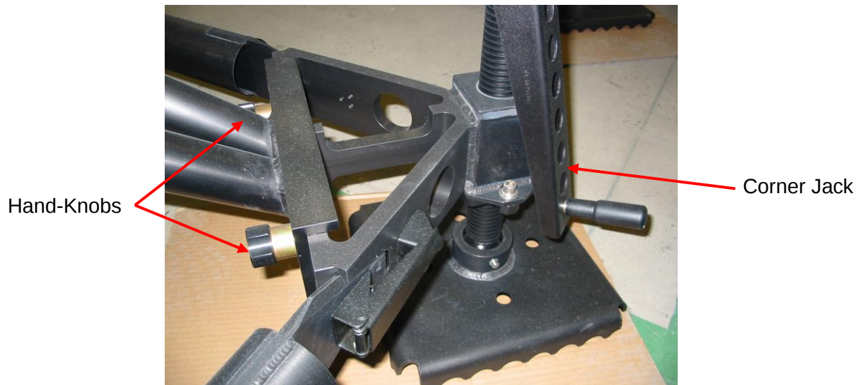
Figure 8. Diagonal Structure Attachment to Corner Jack
