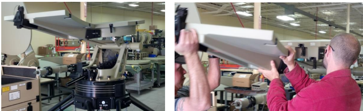
Figure 21b & 21c. Attachment of Reflector Panel 1
