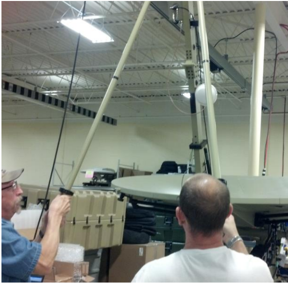
Figure 35a. Lifting the Feed Boom
