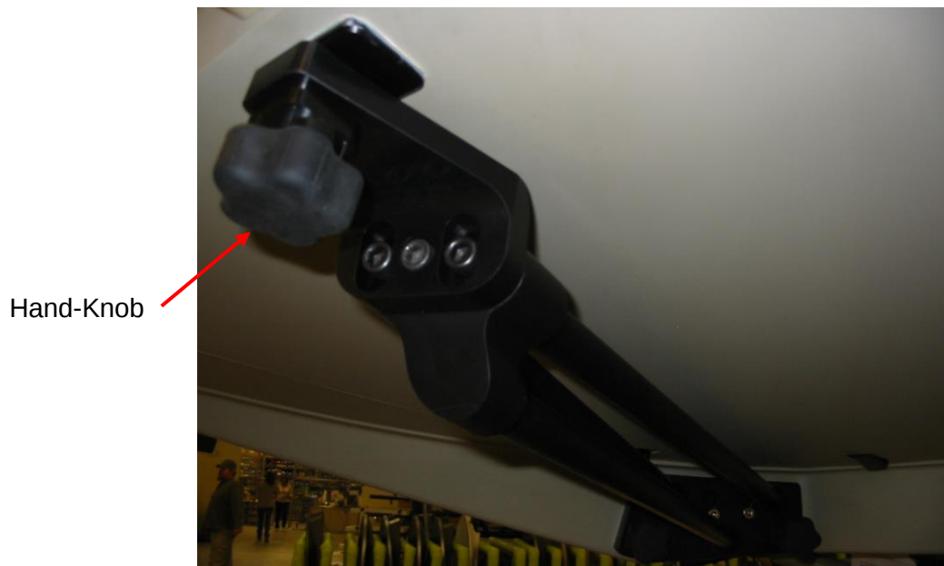
Figure 26. Attachment of Reflector Brace to Panel 2
