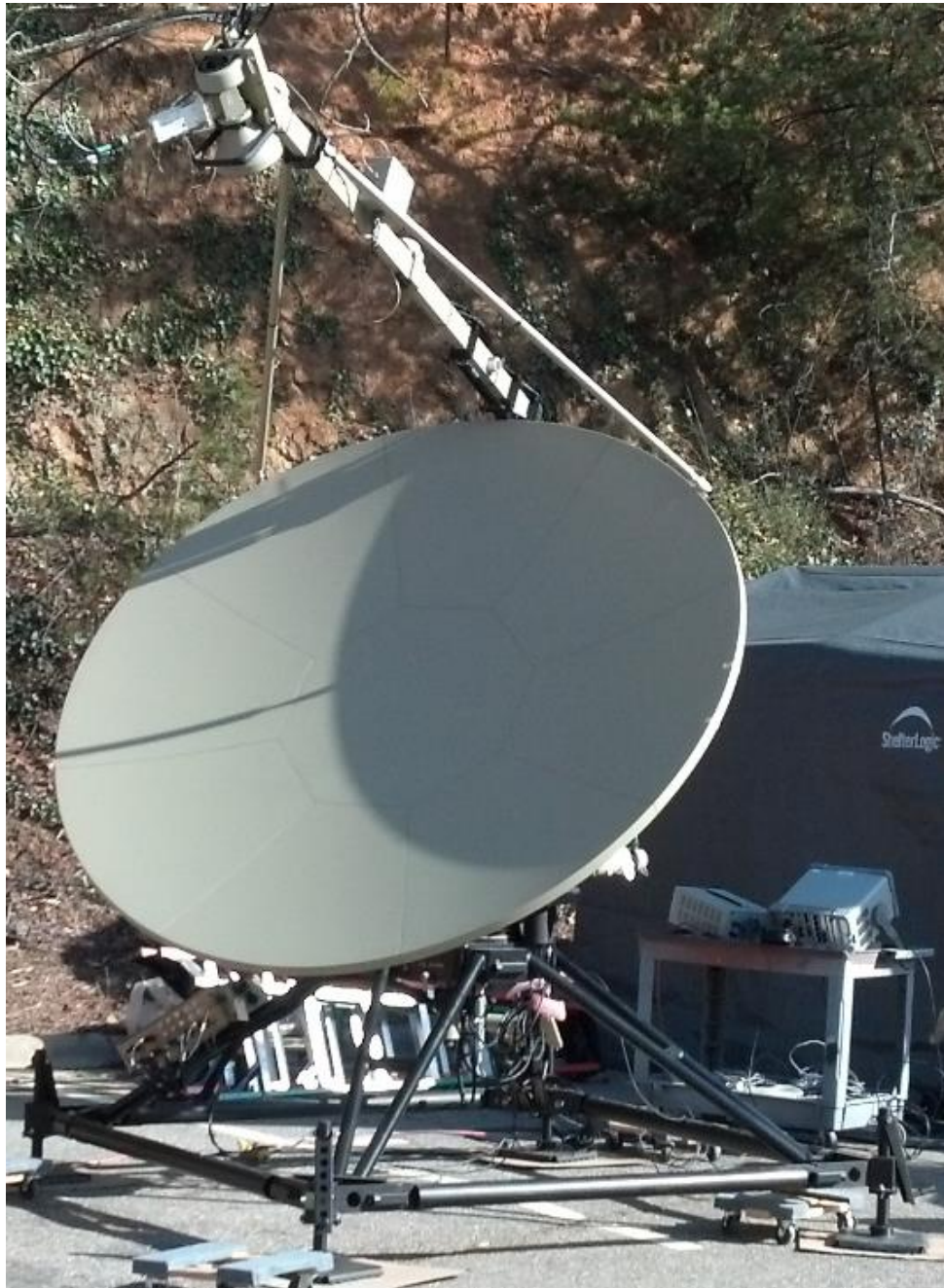
Figure 38. Assembly of Quad-Pod, Positioner, Reflector, and Feed
