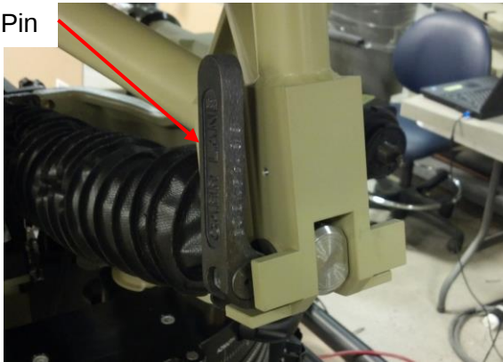
Figure 14. Attaching the Elevation Actuator Assembly
