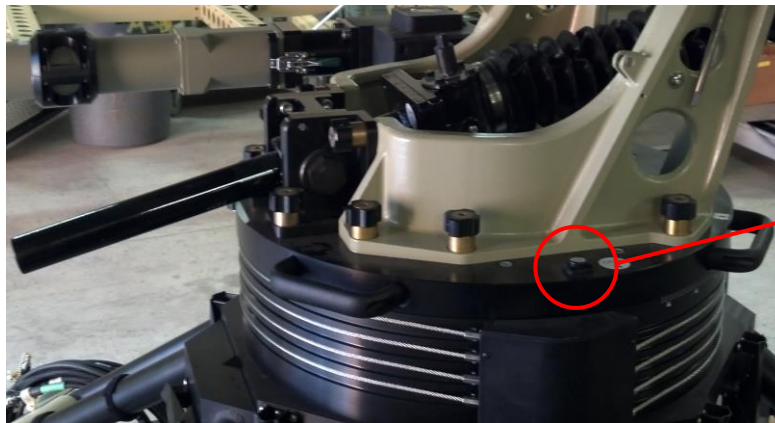
Figure 11. Bubble Level Location on Azimuth Positioner
