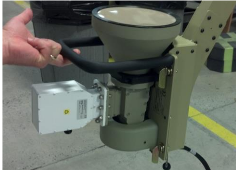
Figure 1. 2460 HW Feed System with Circular Polarization
