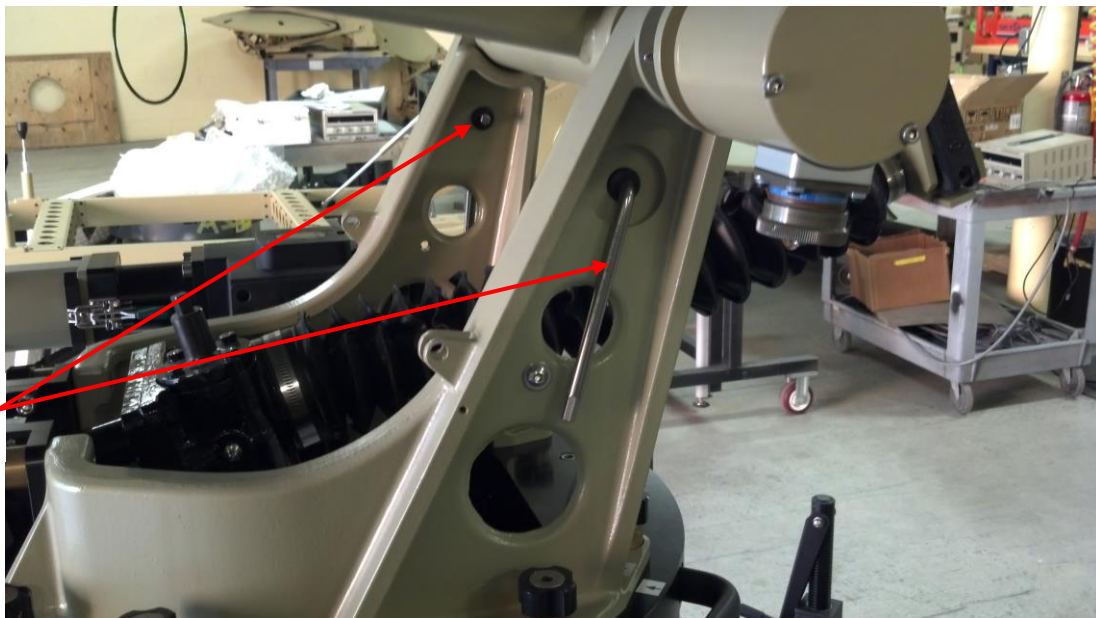
Figure 15. Elevation Frame Allen Wrench Storage Locations
