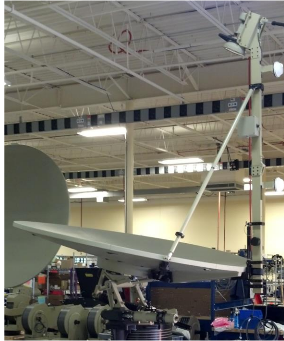
Figure 35b. Feed Boom in Deployed State
