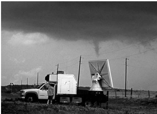
A DOW in operation collecting data near a tornado in the Texas Panhandle in 2003
