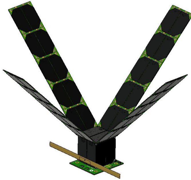
Figure 2. Hatchling Canary in the Deployed Shuttlecock Configuration With Visible Surface Area Between 0.011 \text{ m}^2 and 0.038 \text{ m}^2 .
