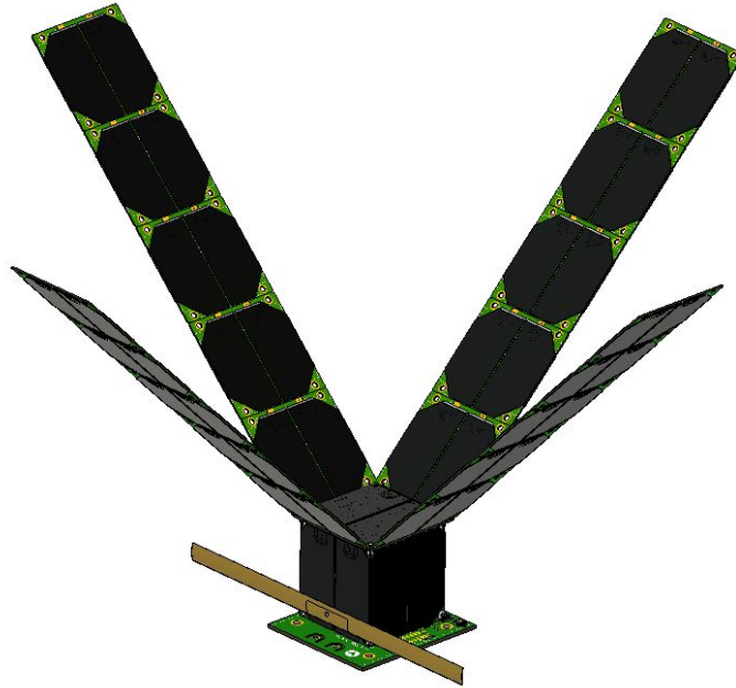
Figure 2. Hatchling Canary in the Deployed Shuttlecock Configuration With Visible Surface Area Between 0.011 m 2 and 0.038 m 2 .
