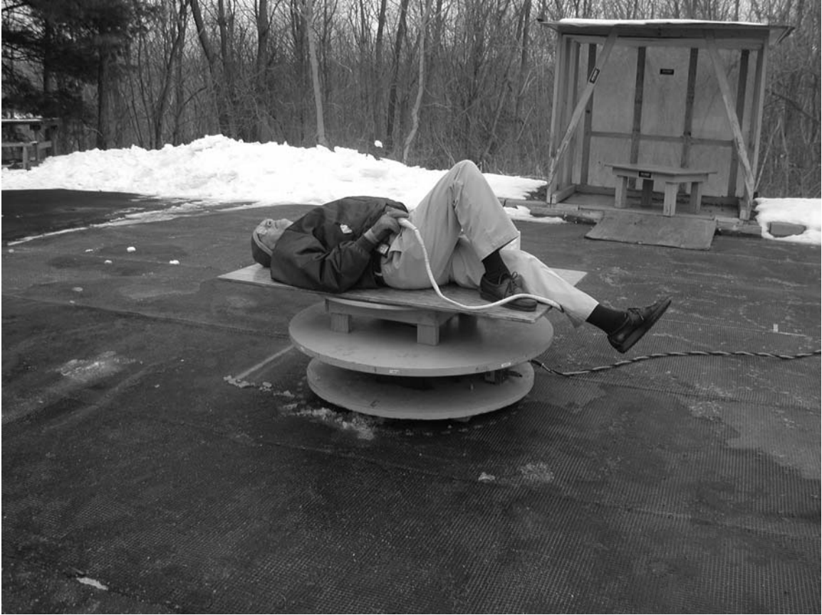
Figure 2. Testing for EMI with a “simulated” patient. The coil (loop) is underneath the blue jacket.
