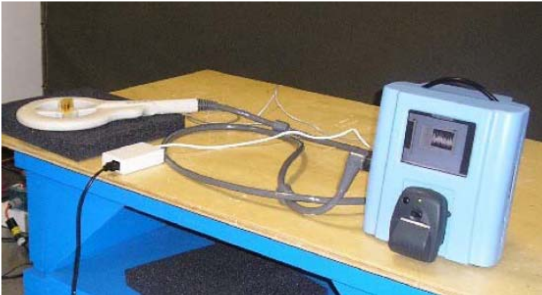
Figure 2. This represents the CardioMEMs version 2 system approved under FCC part 18. The documented frequency range is 30-37.5MHz, but CardioMEMs needs to operate this up to 42MHz for the U.S. clinical trials of the heart failure sensor.
