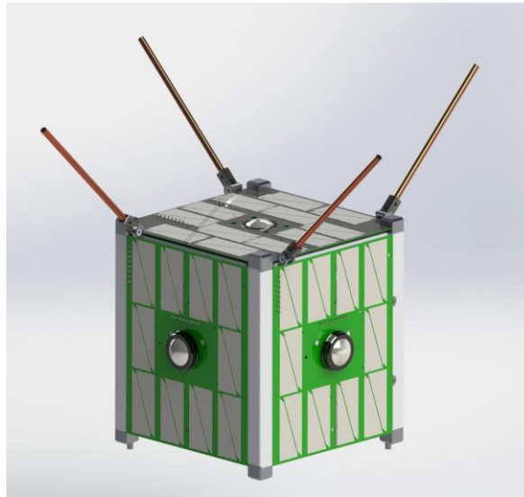
Figure 1. 1U Passive Inspection Cube Satellite Overview
