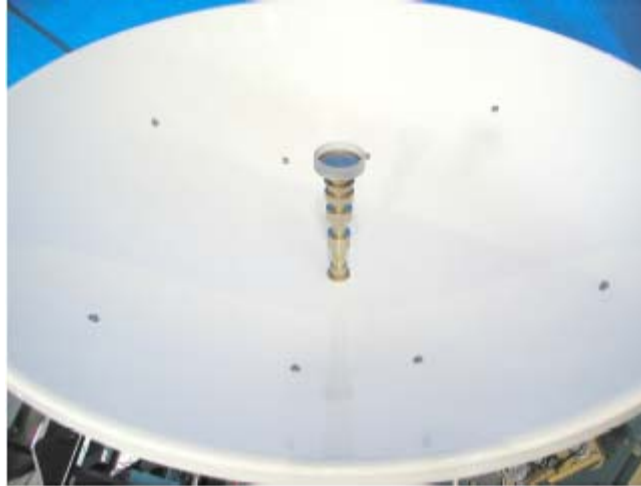
Figure 2. CBBM ESV 0.6 m antenna
