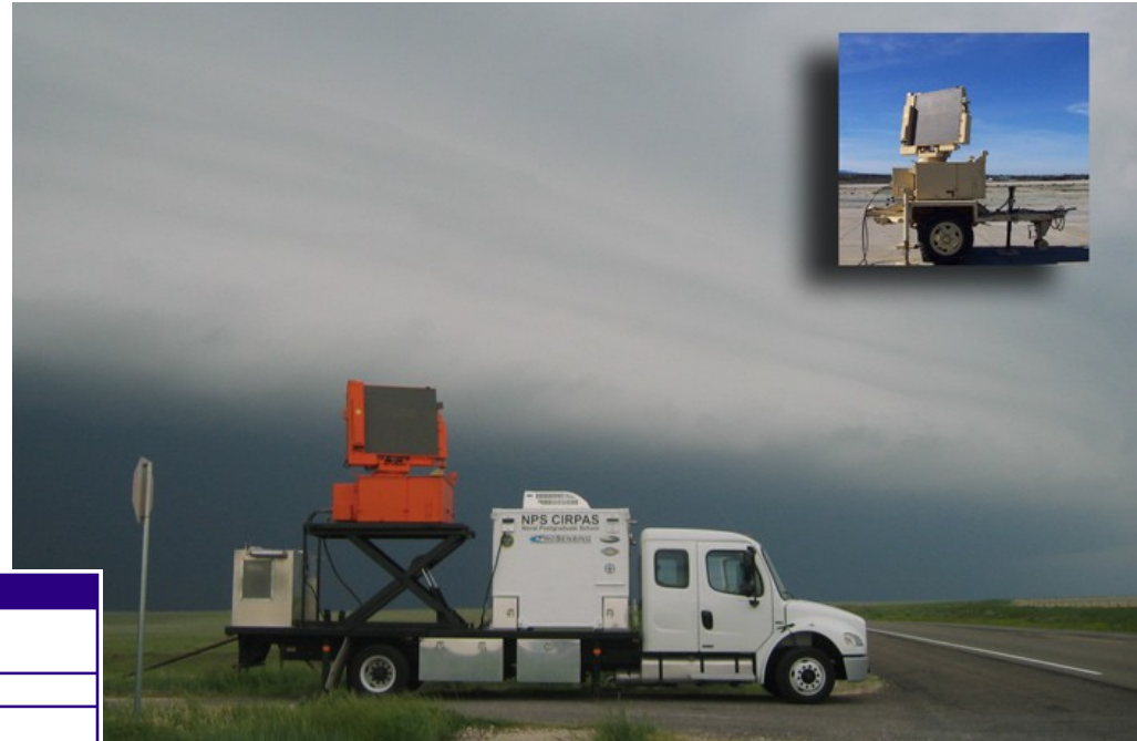
MWR-05XP installation on flatbed truck
