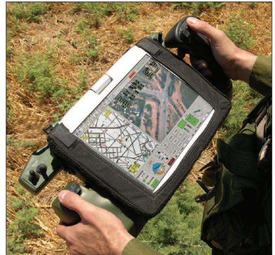
The Orbiter aircraft can be controlled easily using its personal GCS.
