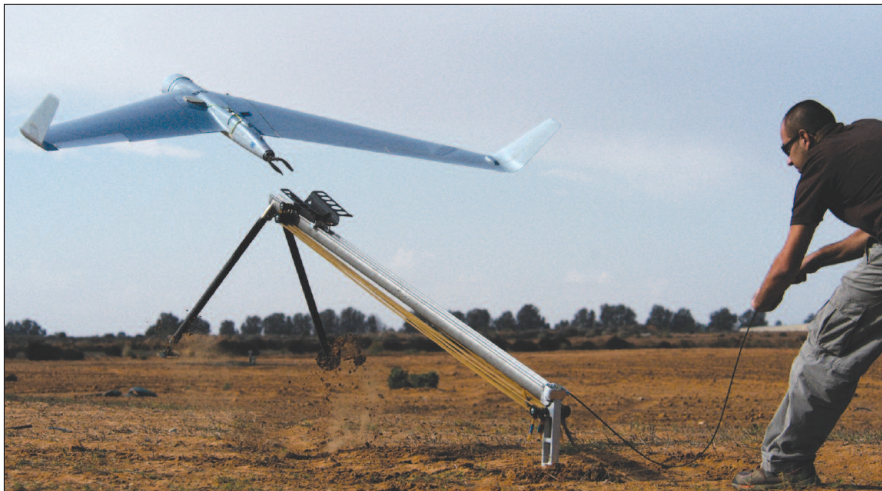
The Orbiter Mini-UAS launches using a catapult that incorporates redundant safety features.
