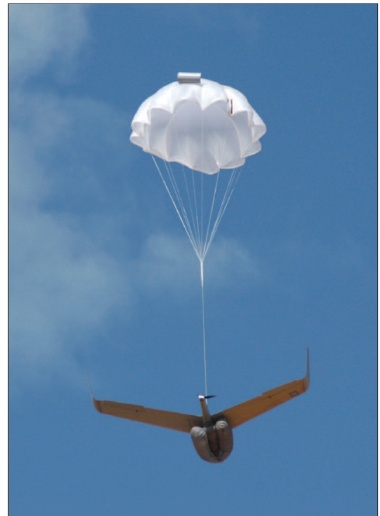
An automatic parachute and air bag recovery system can be deployed virtually anywhere.
