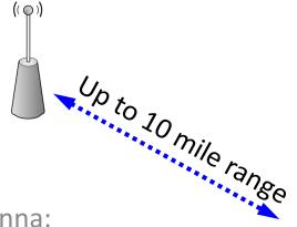
Terminal radio has a directional antenna:
